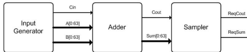
Figure 51. Block diagram of Prefix Adder and its test circuitry
